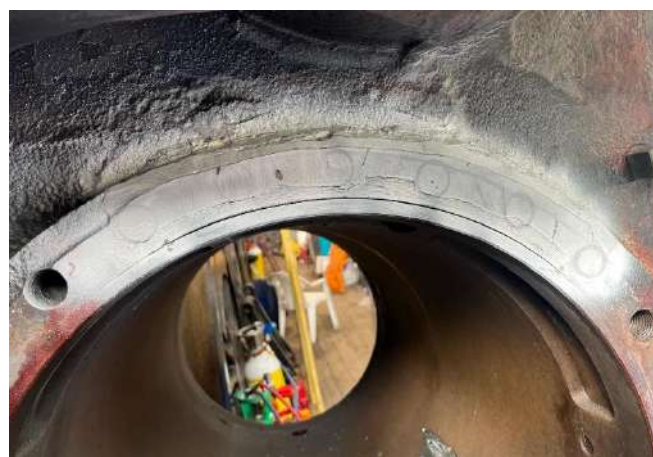
Rebuilt area on front of cylinder (Allan Schoffield)
